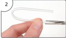
Take a piece of U-shaped tubing. Taper one end by trimming the tube in half lengthways for 4cm. Cut a point on the end
