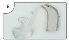
Make sure the mould bends in the right direction as shown
